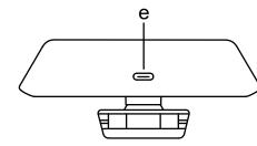
a.Microphone b.Indicator Light c.Ca d.Camera Bracket e.USB Type-C
