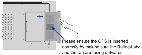
3. Fix the screws or mounting ears and tighten it
