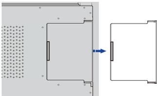
2. Insert OPS PC Module into the panel slot
