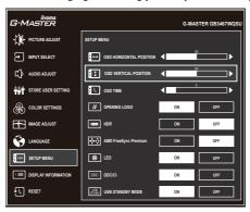
Press the Menu Button and finally the ◀ Button to close the On Screen Display feature. All changes are saved in the memory.
