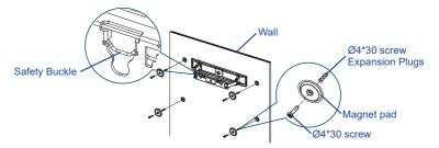
④ Hang the M6 screws into wall mount recesses, press the Safety buckle back, organize display cables into the alignment slots.
