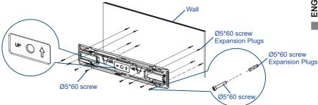
3 Extend the wall mount to maximum and unlock the Safety buckle to observe the alignment of display back cover screws and bracket hook slots.
