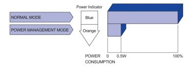
**NOTE** Even when using the power management mode, the monitor consumes electricity. Turn off the Power Switch whenever the monitor is not in use, during the night and weekends, to avoid unnecessary power consumption.
