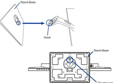
Thumb screw for Stand-Base fixing
