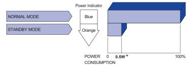
\* USB peripherals and audio equipment are not connected.
