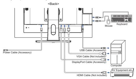
\* VGA cable is not supplied with the monitor. If you use low quality VGA cable, it may cause a result of electro-magnetic interference. Please contact the iiyama Support Centre in your country if you wish to connect the monitor via the VGA input.
