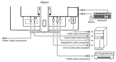
\* DVI dual-link cable is not supplied with the monitor. If you use low quality DVI dual-link cable, it may cause a result of electro-magnetic interference. Please contact the iiyama Support Centre in your country if you wish to connect the monitor via the DVI input.
