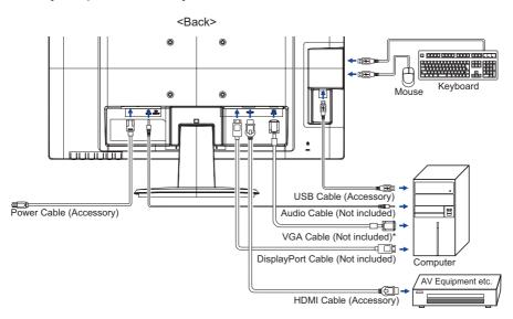
\* VGA cable is not supplied with the monitor. If you use low quality VGA cable, it may cause a result of electro-magnetic interference. Please contact the iiyama Support Centre in your country if you wish to connect the monitor via the VGA input.
