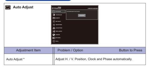
Only Analog Input. For best results, use the Auto Adjust in conjunction with the adjustment pattern. See page 28 for SCREEN ADJUSTMENTS.
