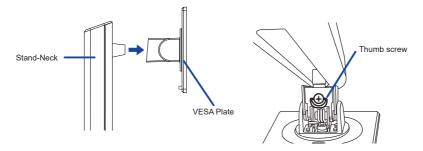
④ Install the Stand-Base to the Stand-Neck and then tighten the 'thumb screw' with the provided screwdriver to secure them.
