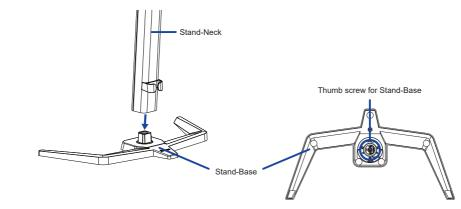
(5) Hold the monitor and install the Stand-Neck to the monitor until it clicks to secure.
