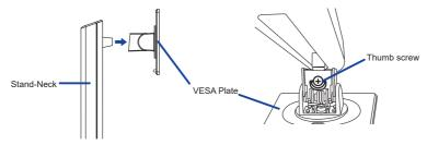
② Install the Stand-Base to the Stand-Neck and then tighten the 'thumb screw' with the provided screwdriver to secure them.
