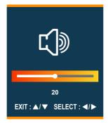
• Mute: Tilting the Joystick [⇔] for about 4 seconds with no Menu displayed. Mute and Unmute are switched by repeating the above Joystick operation.
