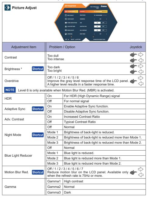
Adjust the Brightness when you are using the monitor in a dark room and feel the screen is too bright.
