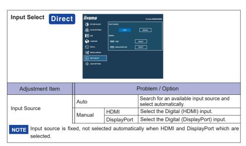
You can skip the Menu items and directly display an option setting screen by using the following button operations.
