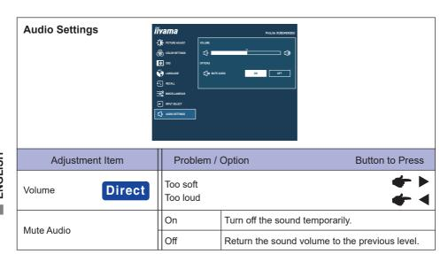
You can skip the Menu items and directly display an adjustment scale by using the following button operations.
