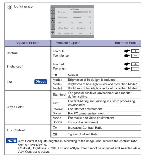
Adjust the Brightness when you are using the monitor in a dark room and feel the screen is too bright.
