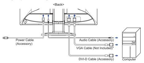
\* VGA cable is not supplied with the monitor. If you use low quality VGA cable, it may cause a result of electro-magnetic interference. Please contact the iiyama Support Centre in your country if you wish to connect the monitor via the VGA input.
