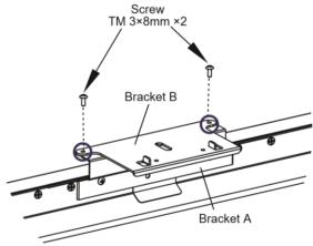
2. Attach the Bracket A to the monitor and tighten those with the screws (TM  $3 \times 8$  mm 2pcs).
