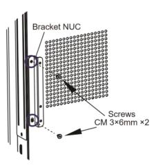
3. Attach your NUC to the Bracket NUC and tighten those with the screws (NUC accessory M4 screw 2pcs).
