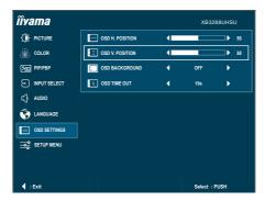
Press the ◀ Button lastly to close the On Screen Display feature. All changes are saved in the memory.
