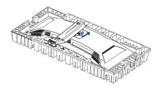
④ Install the Stand-Base to the Stand-Neck and then tighten the 'thumb screw' to secure them.
