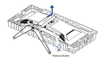
③ Loosen the 'thumb screw' to remove the Stand-Base from the Stand-Neck.
