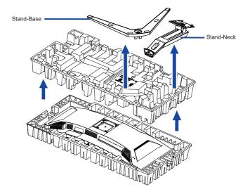
3 Hold the monitor and install the Stand-Neck to the monitor until it clicks to secure.
