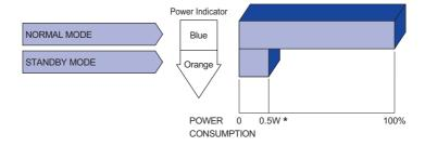
\* USB peripheral and audio equipment are not connected.
