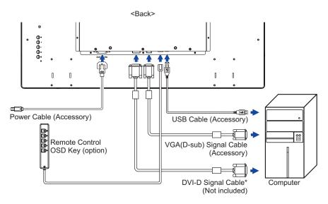
\* DVI-D cable is not supplied with the monitor. If you use low quality DVI-D cable, it may cause a result of electro-magnetic interference. Please contact the iiyama Support Centre in your country if you wish to connect the monitor via the DVI input.
