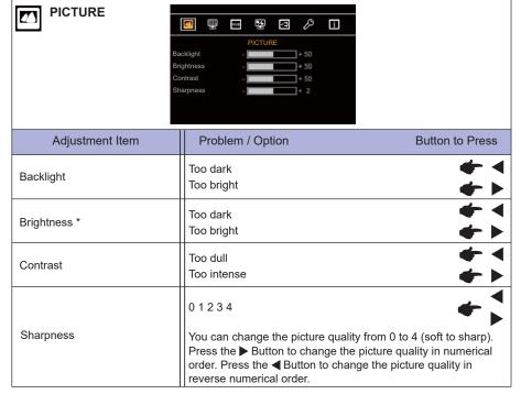
Adjust the Brightness when you are using the monitor in a dark room and feel the screen is too bright.
