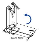
③ Use the 'thumb screw' provided to secure the stand-base to the stand-neck.
