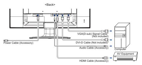
\* Cable is not supplied with the monitor. If you use low quality cable, it may cause a result of electromagnetic interference. Please contact the iiyama Support Centre in your country if you wish to connect the monitor via the VGA or DVI input.
