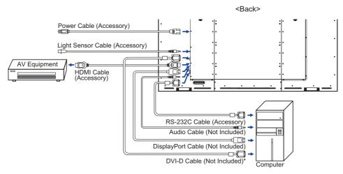
\* DVI-D cable is not supplied with the monitor. If you use low quality DVI-D cable, it may cause a result of electro-magnetic interference. Please contact the iiyama Support Centre in your country if vou wish to connect the monitor via the DVI input.
