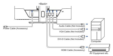
\* Cable is not supplied with the monitor. If you use low quality Cable, it may cause a result of electro-magnetic interference. Please contact the iiyama Support Centre in your country if you wish to connect the monitor via the VGA or DVI input.
