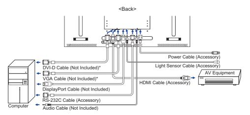
\* Cable is not supplied with the monitor. If you use low quality cable, it may cause a result of electromagnetic interference. Please contact the iiyama Support Centre in your country if you wish to connect the monitor via the VGA or DVI input.
